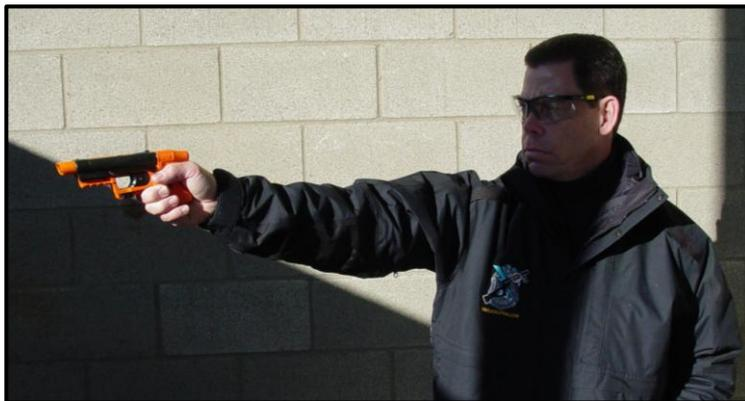
**The JPX Jet Projector did not result in any ignition or heat production.** The thermal imaging recorded a slight drop in temperature at the electrical arc, and no indication of ignition.
